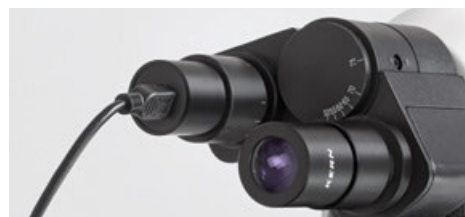
Eyepiece camera fixed into the tube
