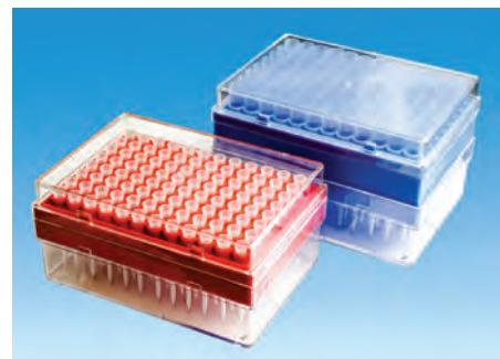
**WITOPET** Filtertips (**sterile**) suitable for all **WITOPET** pipettes, autoclavable
