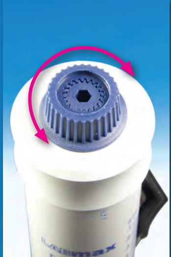
**NEW****Built-in recalibration****Zero loss of reagent**
