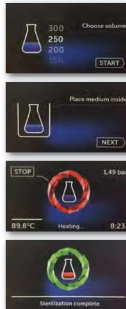
All functions are operated from the touchscreen. The whole sterilization process is shown and every step documented on the micro SD card.
