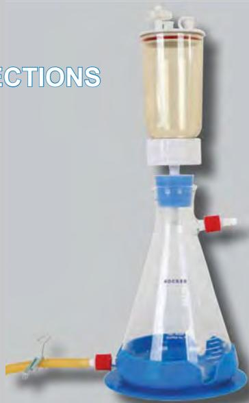
LF 31 - Borosilicate glass receiver flask
