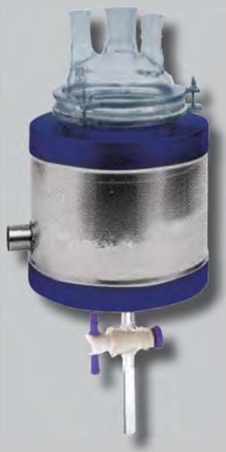
2.000 ml reaction vessel heating mantle
